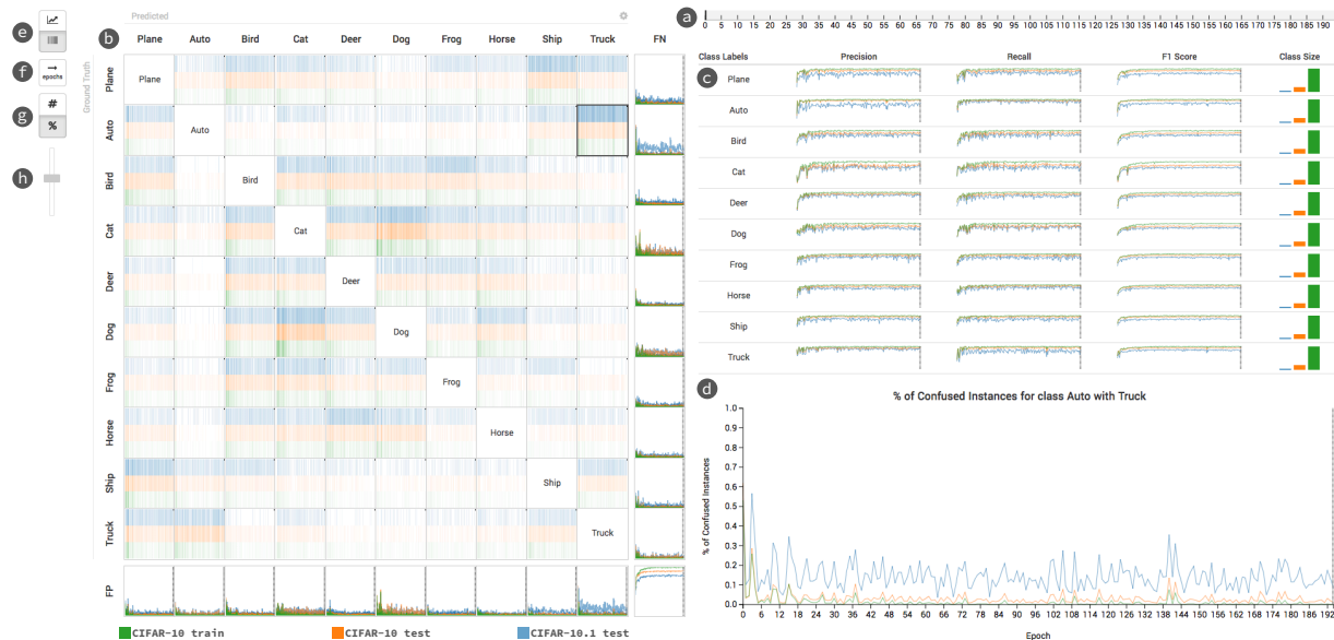
Figure 1: ConfusionFlow consists of three main parts: the timeline (a), the confusion flow visualization (b), and a detail view (c). We show the train set ■ and test set ■ from CIFAR-10 [4] and a recently proposed new test set ■ from CIFAR-10.1 [6]. The line chart (c) shows that the relative number of misclassified images for the selected classes Auto and Truck deviates notably between the original and the new test set, while for the remaining classes the new test set is able to match the distribution of CIFAR-10 (b).
